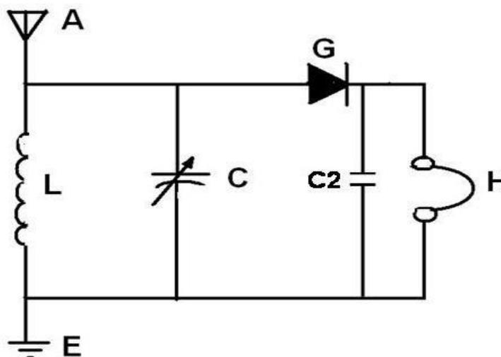
**Fig. #H2** (6 in [10]): Electrical diagram of the "crystal radio" in which instead of galena crystal a germanium diode 1N34 is used. A prototype of that radio was tested and it works for long waves AM. The description of the above radio is provided in the book [6FE], pages 39 to 42, with the electrical diagram of it shown in there on page 41. (Click on this diagram to see it enlarged or to shift it to a different area of the screen.)
